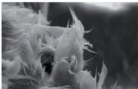
Asbestfasern (Chrysotil) in Bitumen
