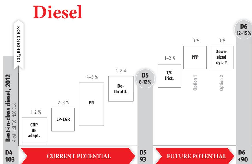
CRP/HF= common rail pressure / hydraulic flow | LP-EGR= low-pressure EGR system
