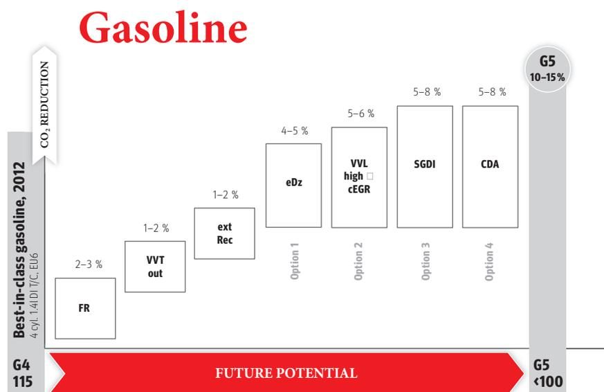
VVT= variable valve timing | SGDI= lean burn | FR= friction reduction engine | eDZ= extreme downsizing
